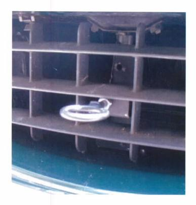
6. Attach the mounting hardware to the License Plate Mounting Bracket. Insert one ½" long 6-32 cap screw into the hole on the back side. The head of the cap screw should have a lock washer and a flat washer under it. The flat washer should be touching the bracket. On the other side of the bracket, push on the nylon screw retaining washer. Repeat for the other hole.
